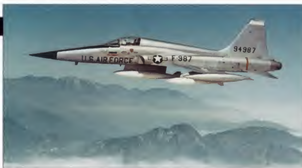
For long-range missions, the Freedom Fighter's wing-tip missile pylons can be replaced with fuel tanks.
